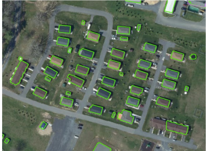
Figure 5. Structures destroyed during or following WV's 2016 flood ( left ) present only in Microsoft's dataset, captured using pre-2016 imagery. Structures constructed post-flood, present only in WVGISTC's dataset, created using 2020 aerial imagery ( above ); White Sulphur Springs, WV
